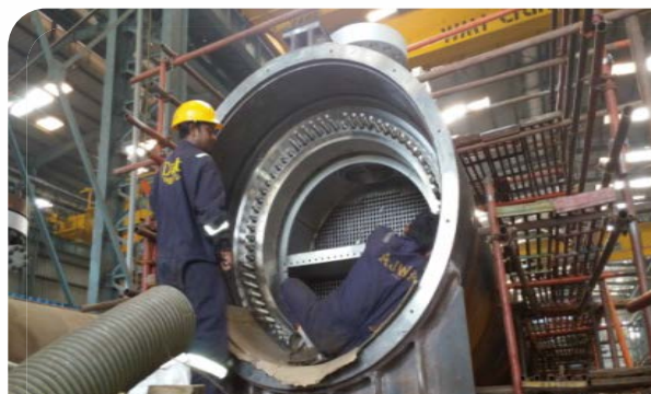
Breach Lock exchangers Size: 1.6 metre OD, MOC: 2.25Cr, 1.0Mo, SS347 weld overlay.
