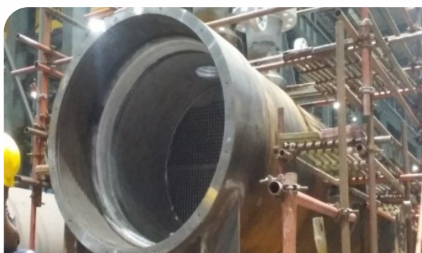
Heat exchangers- Ethylene Fractionator 380 MT, 5000 mm shell diameter and with 15000 no of tubes, 6500mm length.
