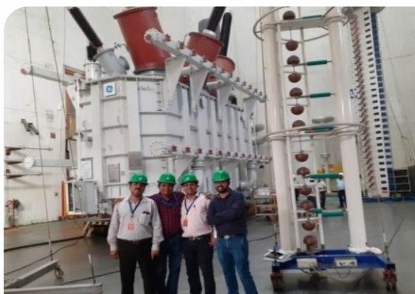
3-Phase, 400/66 KV, 250 MVA Power Transformer.
